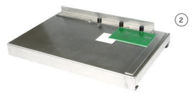
3 Lay the stencil over the PCB and using the magnets, fix it in position on the folding hinge.
